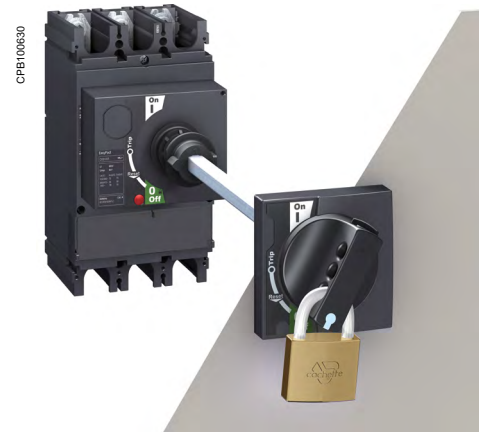
EasyPact EZX400 with an extended rotary handle installed at the back of a switchboard, with the keylock option and key.
