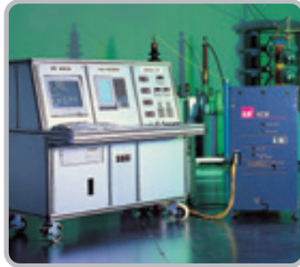
Characteristics Test / VCB Characteristics Test
