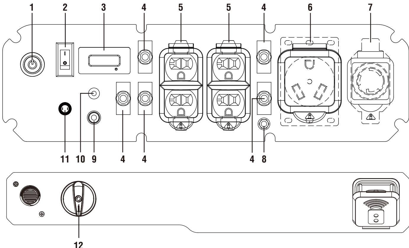
**1. Push-Button START/STOP:** Push once to automatically start the engine. Push again to stop the engine.
