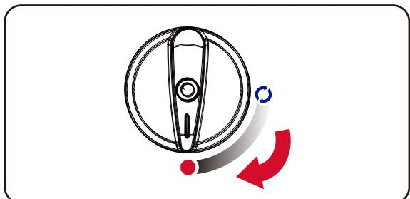
4. Turn off the battery switch to "OFF" (O) position.
