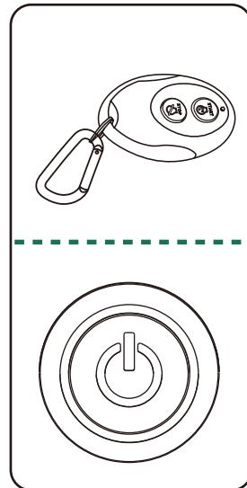
2. Push STOP on the remote start key fob for 3 seconds.
