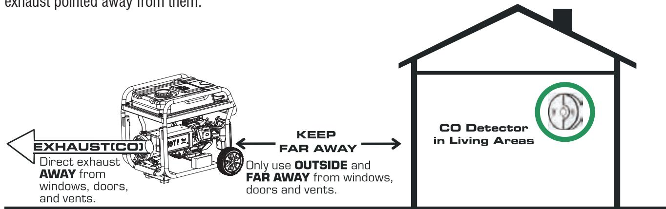
However, if the generator misused and operated in a location that results in the accumulation of CO inside an enclosed or partially enclosed space, CO WATCH-GUARD automatically shuts off the engine and notifies the user of what has happened and directs the user to read the instruction of CO WATCH-GUARD Action Label for steps to take.
