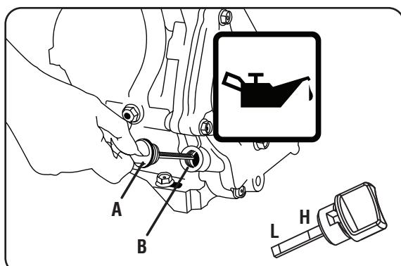
The engine is equipped with a low oil shut-off and will stop when the oil level in the crankcase falls below the threshold level.
