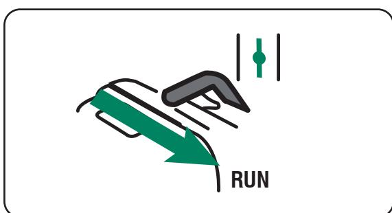
9. Allow generator to run at no load for few minutes upon each initial start-up to permit engine and generator to stabilize.
