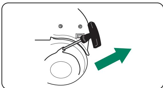
8. Do not over-choke. As soon as engine starts and warms up, move the choke lever to the “**RUN**” position.
